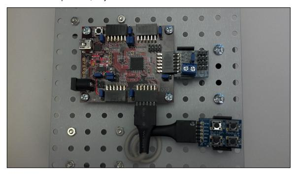
10. Connect the right servo to J4 and the left servo to J5 on the PmodCON3. The white cable must be connected to the pin labeled "SIG".
