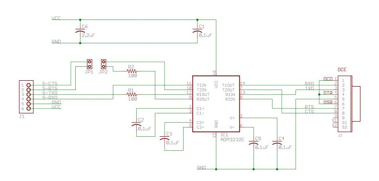
Note: This module is wired as a DCE. Connect to a DTE using a straight through cable. Data transmitted from a DCE to a DTE is on the signal named RXD Data transmitted from a DTE to a DCE is on the signal named TXD J1-Pin 3 is an output. It carries data received from the DTE J1-Pin 4 is an input. It carries data transmitted to the DTE
