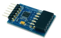
Pmods<sup>™</sup> are small I/O interface boards that offer an ideal way to extend the capabilities of programmable logic and embedded control boards. They allow sensitive signal conditioning circuits and high-power drive circuits to be placed where they are most effective - near sensors and actuators.
