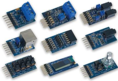
Pmods™ are small I/O interface boards that offer an ideal way to extend the capabilities of programmable logic and embedded control boards. They allow sensitive signal conditioning circuits and high-power drive circuits to be placed where they are most effective - near sensors and actuators.
