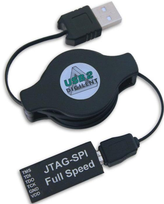
Every JTAG-USB Full Speed module is given a unique serial number. The Adept software uses this serial number to connect to the device.
