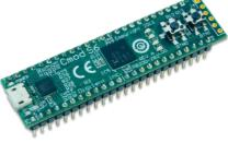
also includes a programming ROM, clock source, USB programming and data transfer circuit, power supplies, and basic I/O devices. There are 46 FPGA I/O signals that are routed to 100-mil-spaced through-hole pins, making the Cmod S6 well suited for use with solderless breadboards. At just .7" by 2.6" inches, it can also be loaded in a standard socket and used in embedded systems.
