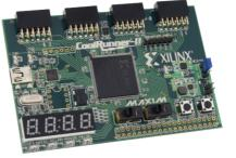
oscillator, several I/O devices, and a USB2 port for board power and CPLD programming. The board also includes five expansion connectors that make 64 CPLD signals available to external circuits.
