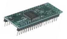
convenient 600-mil, 40-pin DIP package. Cmods are ideally suited for breadboard or other prototype circuit designs where the use of small surface mount packages is impractical.
